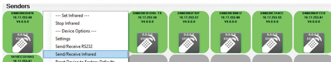
FIGURE 4-36. MCX CONTROLLER INFRARED – SENDING/RECEIVING IR DATA
