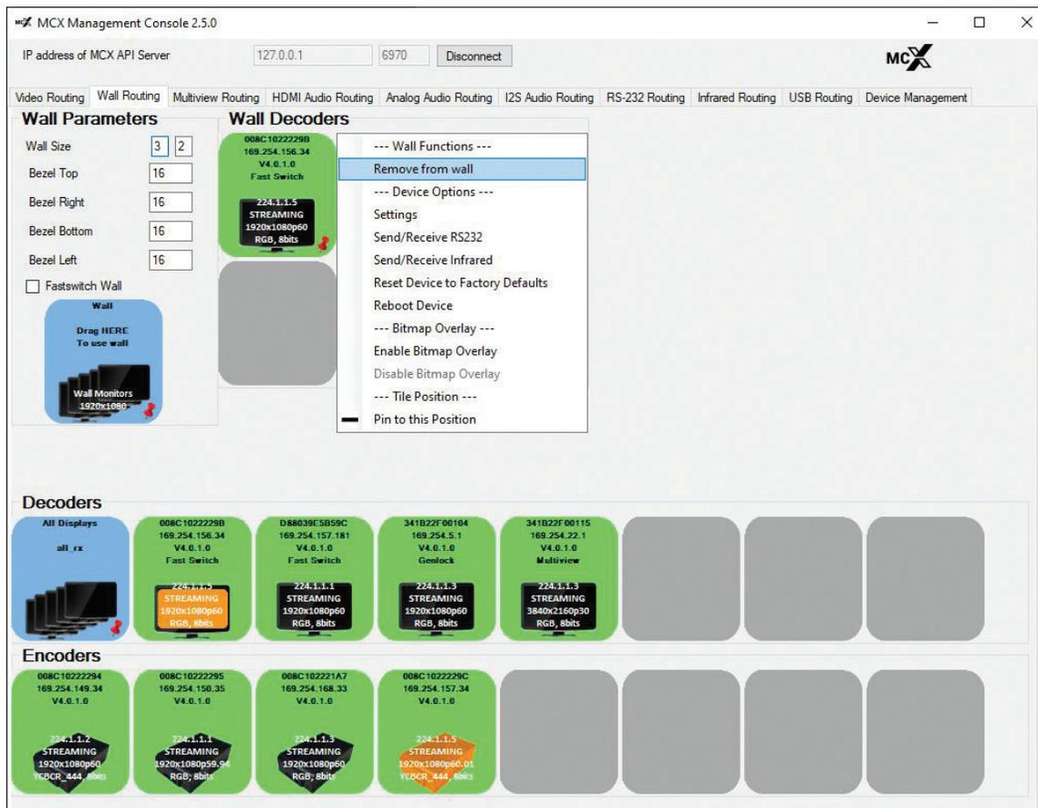
FIGURE 4-9. REMOVING A DECODER (RX) FROM A WALL
