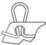
Figure 4-7. Create a loop from the power cable and feed it through the hole at the top front of the divider.
