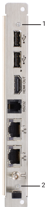
FIGURE 2-8. STATUS LEDs ON CPU BOARD (ACX288-ADCTL)
