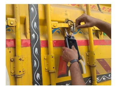
JIDO has a smart lock system, which can only be opened by an authorized person who has its key. In the event of unauthorized opening of the container, opening of the container in a place not intended for loading or unloading cargo, or any attempt to tamper with the container or JIDO, an alert goes out immediately to Indian Railways with all the details, including the location and road train number.
