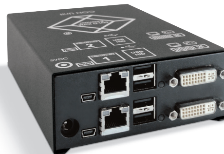
DKM COMPACT TRANSMITTER CATX SINGLE DVI, USB HID PLUS DIGITAL AUDIO (ACX1T-12D-C)
